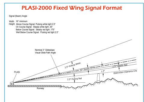
The PLASI-2000 and HELI-PLASI visual approach aids are FAA certified and listed under specification L-883 Generic Visual Glideslope Indicators. The system has the range, brilliance, and angular coverage that is required per FAA regulation AC-5345-53C.
